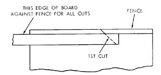
Turn workpiece over end for end . . . keep same edge against fence when making successive cuts.
